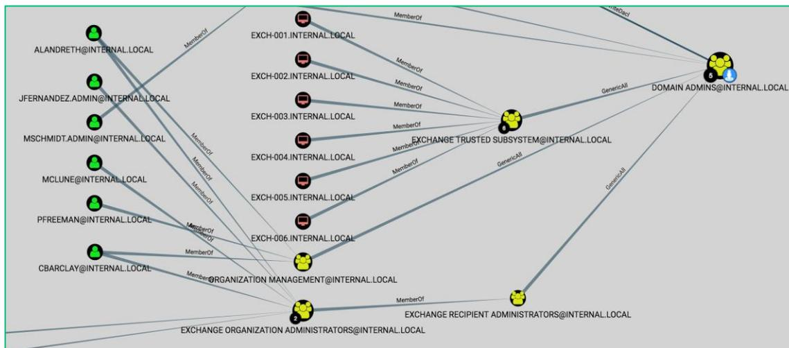
***Above: Detail of the previous figure, showing several computers belonging to the security group “Exchange Trusted Subsystem”, which in turn has the “GenericAll” (or Full Control) relationship to the “Domain Admins” group.***
