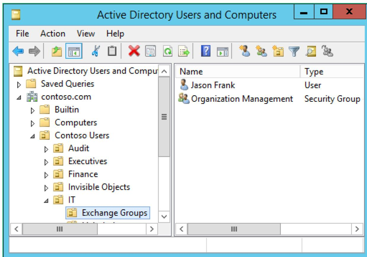
*Above: The “contoso.com” domain contains the OU “Contoso Users”, which contains the OU “IT”, which contains the OU “Exchange Groups”, which contains the user “Jason Frank”.*
