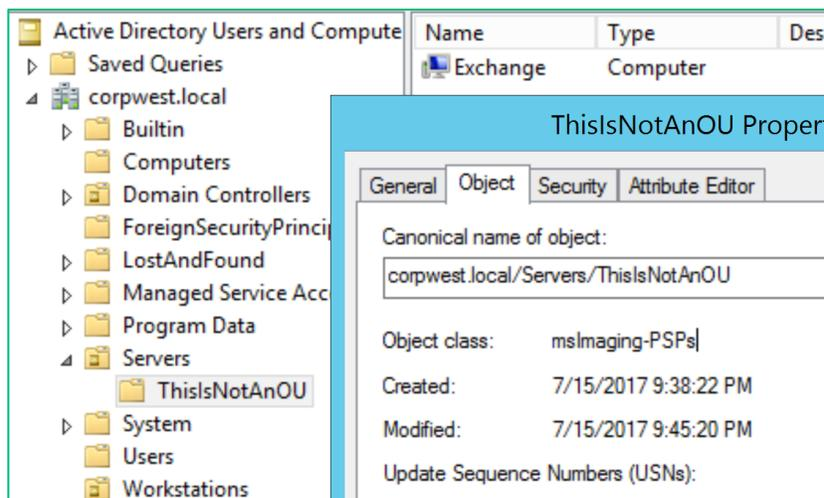
**Above: 1) Compromised IT admin adds an mslmaging-PSPs object "ThisIsNotAnOU," a type of container, to an existing OU and moves the computer "Exchange" from the Server OU into it.**
