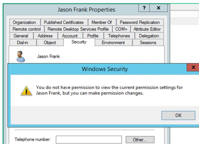
***Above: When clicking the “Security” tab on the user object in ADUC, the above alert is displayed, informing the user that they do not have permission to view permissions on the object.***
