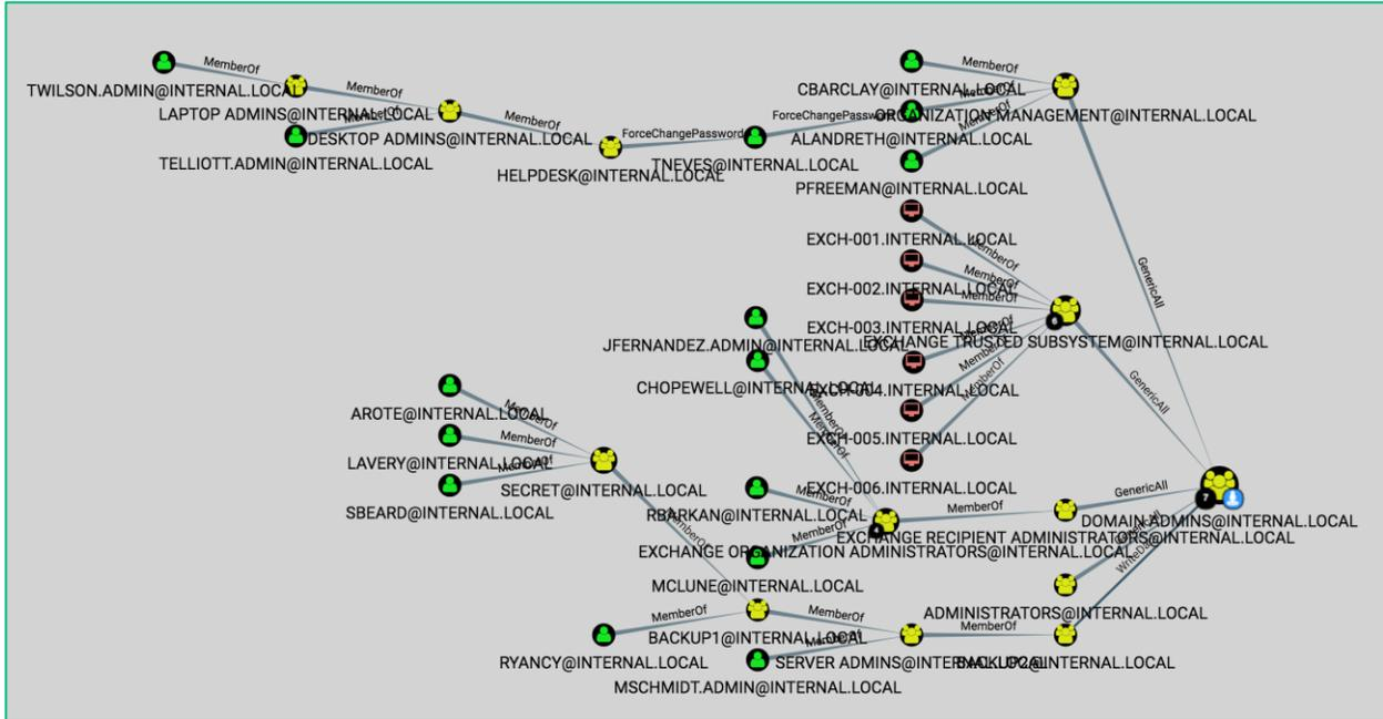
*Above: The BloodHound interface displaying the objects with a transitive object control attack path to the “Domain Admins” group. These are principals which may execute an ACL-enabled attack path to take over the “Domain Admins” group, without a derivative local admin style attack.*
