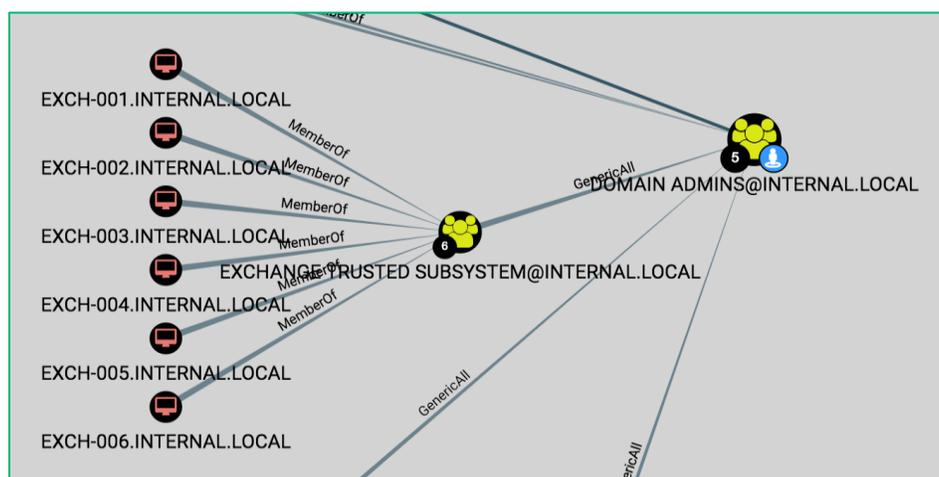
***Above: A typical scenario in many enterprise networks: the Exchange Trusted Subsystem, with all Exchange computer objects as members, has full control over the Domain Admins group.***
